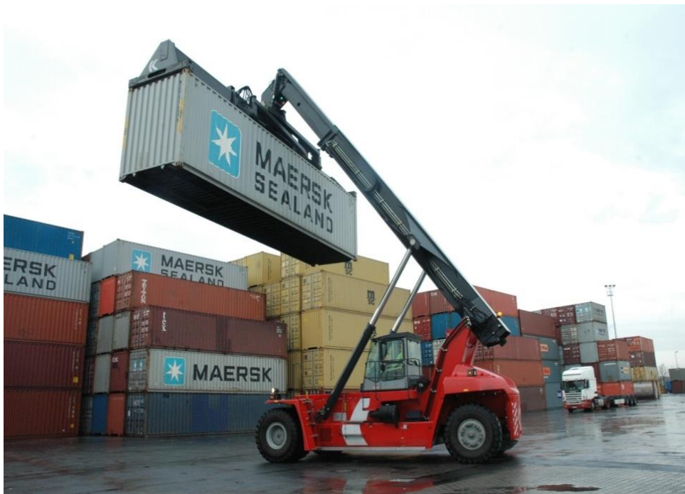
Figure 11. Reach Stacker (5 High, 42-ton Capacity)
